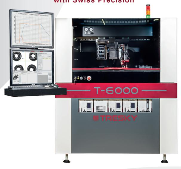
The **T-6000L** Die Bonder is a fully-automated all-purpose system for R&D, pilot and medium size production.
