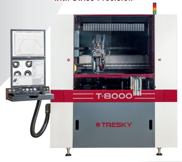
The T-8000 Die Bonder is a fully-automated all-purpose system for R&D, pilot and medium size production. Fully built on granite, equipped with linear motors and 0.1μm resolution glass scales, enable a precision of 5μm. A force range of 10g to 25kg, combined with the large working area of 500 x 450mm and wafer handling up to 12", open a wide range of applications. With numerous available options,
