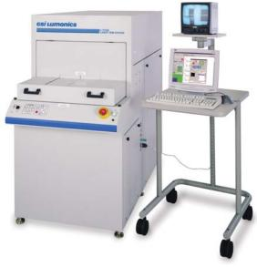
An advanced new platform ideal for trim and test of thick film components and circuits, including PCBs, SMT components, and hybrids.
