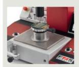
Work area 40 x 40 mm Z-Stroke 40 mm max. part size XY 200 x 150 mm
