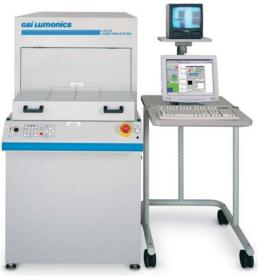
An advanced new platform ideal for trim and test of thin film resistors, resistor networks, and other thin film applications.
