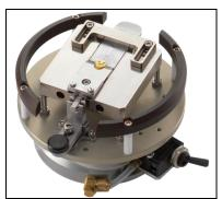
TO workholder with mechanical clamping
