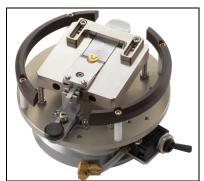
TO workhoder with mechanical clamping
