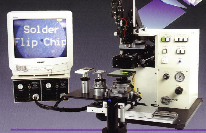
Semiconductor Equipment Corporation's Model 850 is a versatile, semi-automatic placement system for flip chips, chip scale devices and bare die. The system is intended for low volume production and development projects requiring accuracies of +/- 12 microns. A typical application consists of a cycle in which devices are picked up from a waffle pack, dipped into flux and then placed on a substrate.
